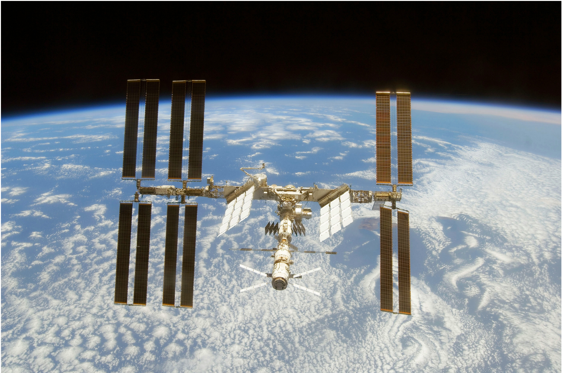
International Space Station (ISS) with deployable solar arrays. Attitude control using gyros.
