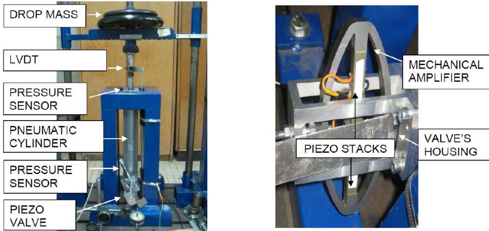
Figure 7 Experimental stand and piezo-valve.
