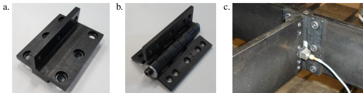
Figure 9. Detailed view of the nodes: a. rigid node, b. pinned node, c. mounted rigid node with an installed accelerometer.
